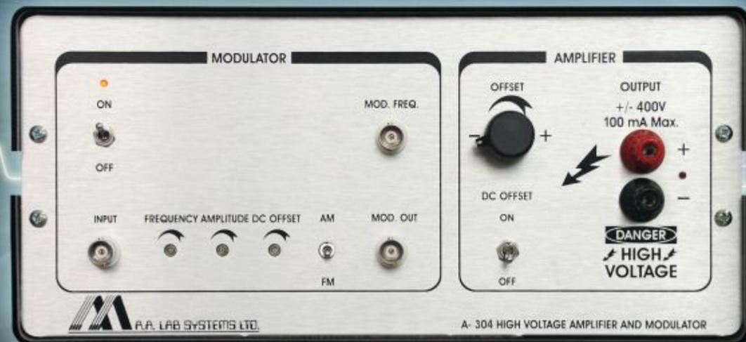
The A-304 piezo Driver/Piezo Amplifier is a high Voltage, high speed Piezo Driver / Linear Amplifier combined with a wide band AM/FM modulator.
