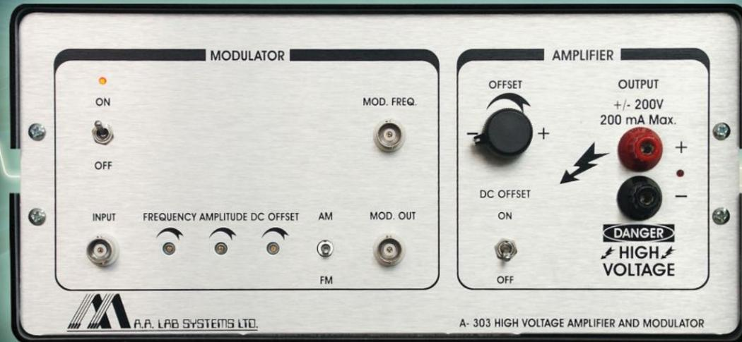
The A-303 piezo Driver/Piezo Amplifier is a high Voltage, high speed Piezo Driver / Linear Amplifier combined with a wide band AM/FM modulator. It was especially designed as a Linear Amplifier / Driver for PIEZO Electric Actuators (also known as "Piezo Amplifier"), stacks, piezo sheets, bimorph elements and other devices. It may be also used as a general purpose High Voltage amplifier for medical applications (for example, as electrode driver for Neurology).
